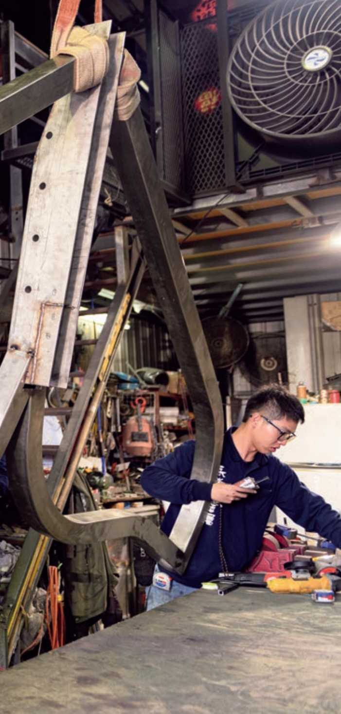
Zeng Wen-chang and employees in his ironworks shop work on a bus stop shelter in the shape of a whale tail (left). A young worker welds components of the bus stop shelter (above).
